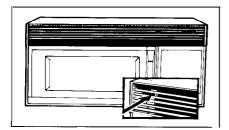
The disposable charcoal filter should be replaced when it is noticeably dirty or discolored (usually after 6 to 12 months, depending on hood usage). Order Part No. WB02X4267 from your GE supplier. DO NOT CLEAN THIS FILTER. DO NOT OPERATE YOUR HOOD WITHOUT ALL THREE FILTERS IN PLACE.
